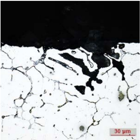
Figure 4: Microstructure of the sample after 480 h in a corrosive environment.
