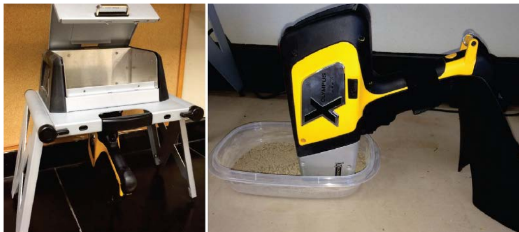
Figure 3: Hands-free pXRF operation using a hooded sample stage for special applications (left) and a bipod stand (right).
