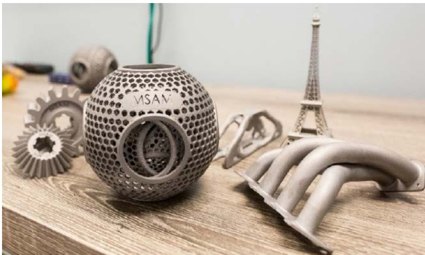
Figure 2: Complex parts made by AM. The spherical nest has three spheres inside.
