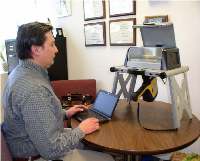
Figure 1: Scanning a sample for elemental characterization with a pXRF spectrometer operated in benchtop mode.
