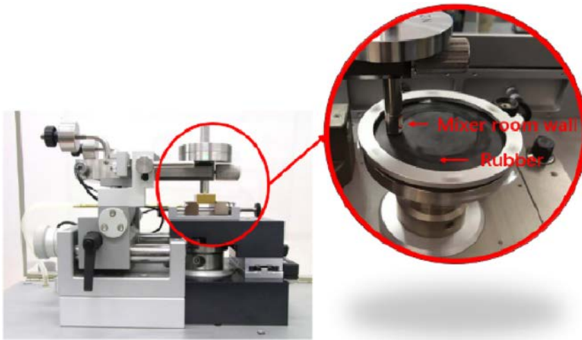
Figure 2: Configuration of the CSM wear test device
