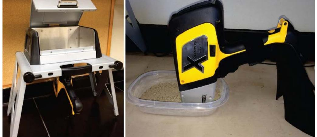
**Figure 3:** Hands-free pXRF operation using a hooded sample stage for special applications (left) and a bipod stand (right).
