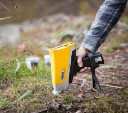
Five XRF Accessories for Mining and Geochemical Analysis Field Kit Handheld XRF analyzers can provide immediate, onsite elemental measurements for a range of mining and geochemical analysis applications, including mineral exploration, ore grade control, and environmental monitoring.
